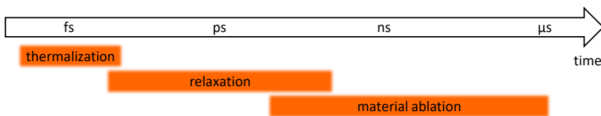
Figure 9: Typical time scales during ultrashort pulse laser material interaction with metals.
