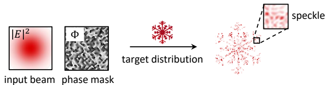
Figure 4: Phase-only beam shaping cannot control wave front and amplitude in the beam shaping plane and a speckle pattern overlays the target structure.
