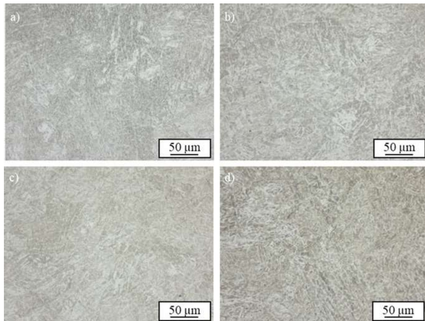
Fig. 10.3 Etched cross-section of the top regions for a unmodified Bainidur AM, b 0.3 wt.% C, c 0.35 wt.% C, and d 0.4 wt.% C
